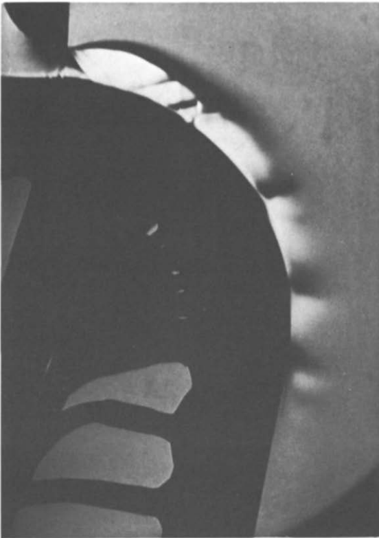
Figure 6 Schlieren, P_a/P_0=0.370 , slot=4 mm
